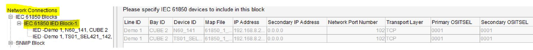
Using the Loader, you can create the client configuration that identifies the devices, points and reporting and polling information required to setup the communications between the IEC61850 compliant server devices and the MCP device.
