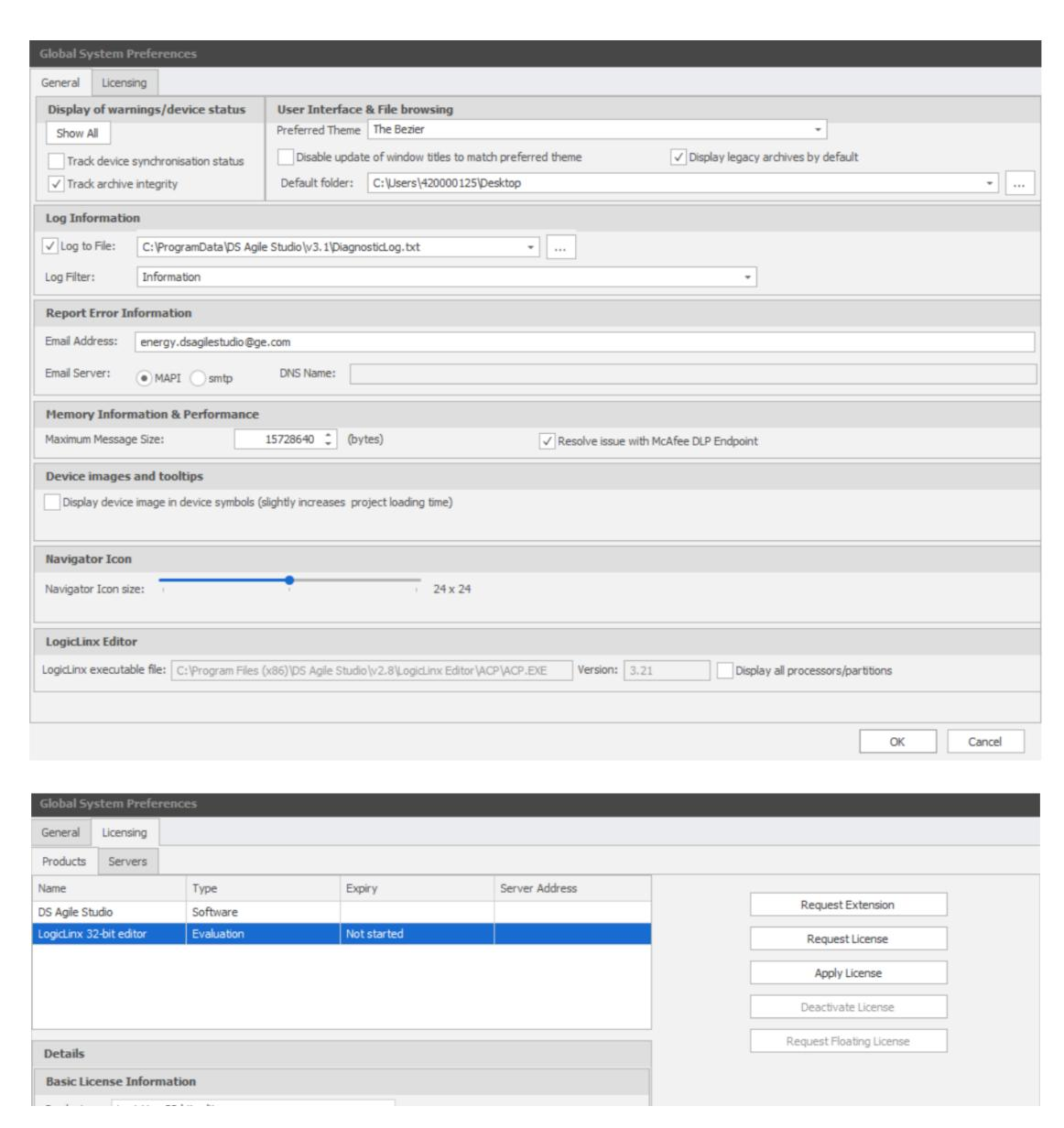
Selecting the option "Display device image in device symbols" slightly increases project loading time.
